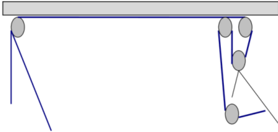
Diagram A. Split tail mainsheet attached to aft pad eyes
