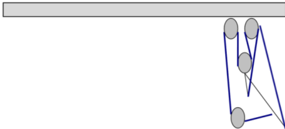
Diagram B. Split tail mainsheet and bridle attached to mid-boat pad eyes
