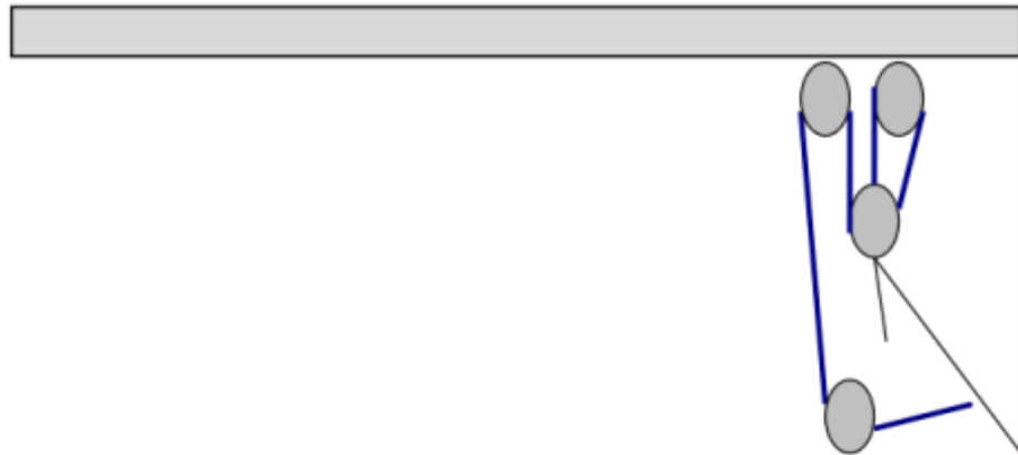
Diagram C. Mainsheet attached to block on mid-boat bridle
