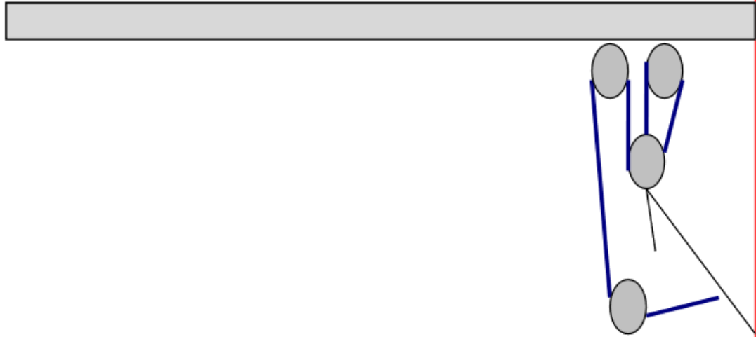
Diagram C. Mainsheet attached to block on mid-boat bridle
