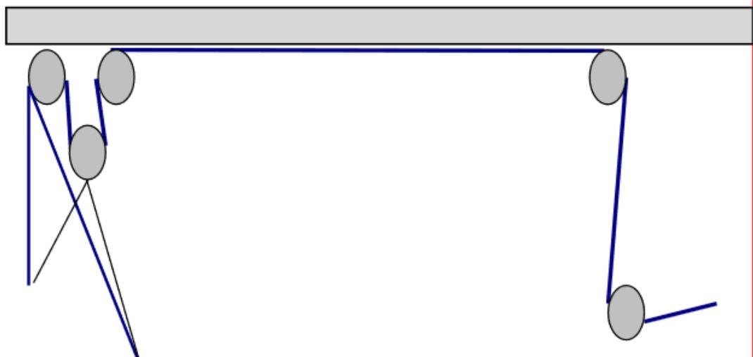
(b) Bridle: The mainsheet must run through a turning point attached to a bridle. The bridle may be of any length but may not be adjustable while racing. The bridle must be attached to either:
