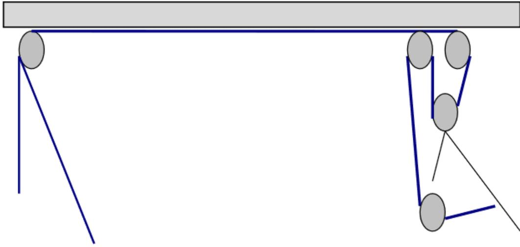
Diagram B. Split tail mainsheet and bridle attached to mid-boat pad eyes
