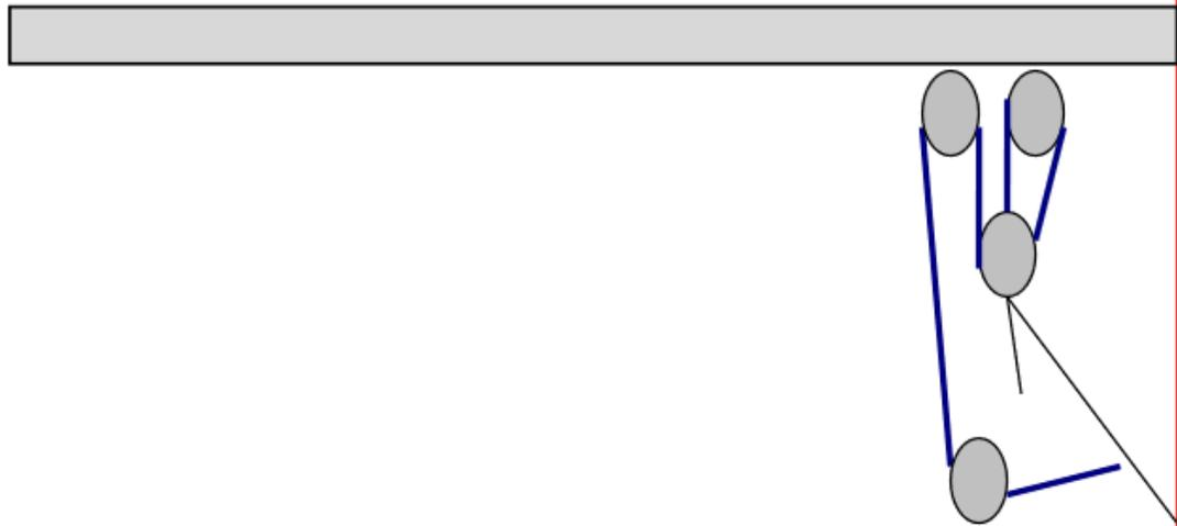
Diagram D. Split tail and bridle attached to aft pad eyes
