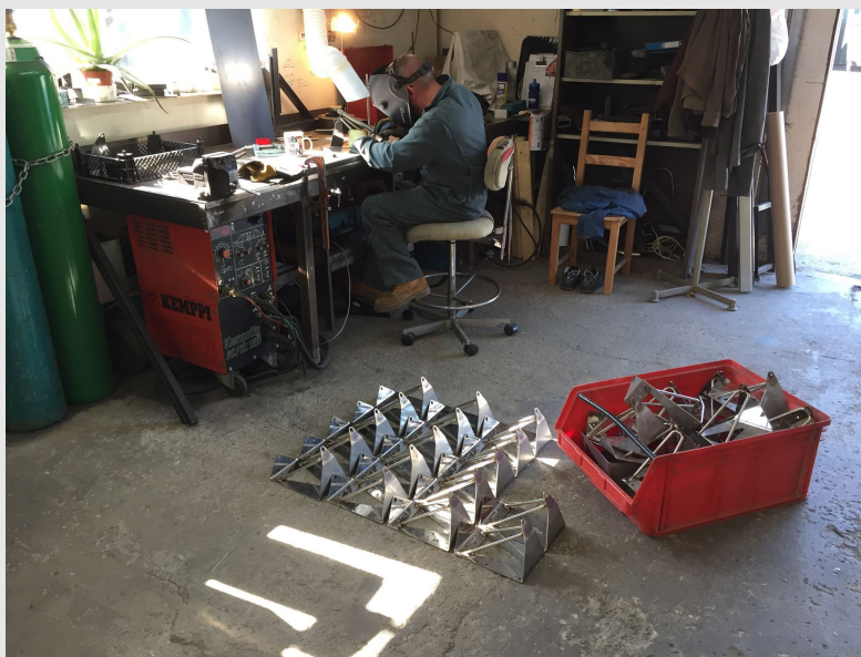
VB2 brackets being welded in the UK.
