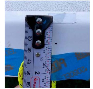
**Step 2**. Mark where to drill through the solid fiberglass gunwale. Shown here is a point about an inch down to get a clean hole all the way through.
