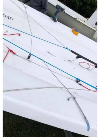
Measuring from the cockpit floor to where the mainsheet turns on the bottom of the block, a height of about 25.5" seems to be a good starting place assuming max headstay length, max aft in the mast step, and North or Doyle sails. Of course other sails and mast setups may require a different dimension.
