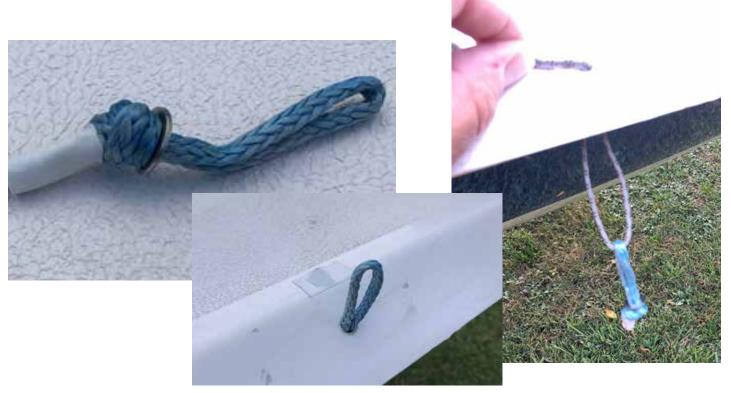
Step 4. Attach a loop to which the aft bridle will connect. Shown here is 3/16's 12-strand spectra.
