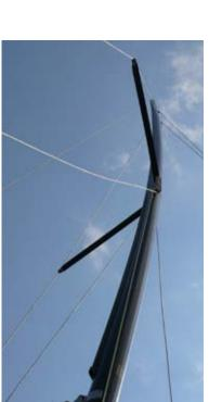
The GNAV is engineered to push down on the boom and forward on the mast, controlling mainsail leech tension. The Aluminum GNAV tube should be of max length permitted by the class, 1280mm (50.4"). With a maximum length GNAV, the point of loading is moved aft along the boom, decreasing boom compression loads and gooseneck sheer loads, while maintaining optimum mainsail leech tension. A Harken or Ronstan ball bearing car system further improves efficiency.
