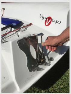
As the vertical rudder orientation is expected to generate highe hardware, Rondar is only building the new gudgeon plates with 10mm bearings for the stronger 10mm pintles. The upside is that these are a wearing part, so the smaller 8mm pintles would have to be replaced at some point anyway. Boats with sail numbers #224 or higher came with 10mm diameter rudder pintles and should order the "A kit" (\$160 / £120).
