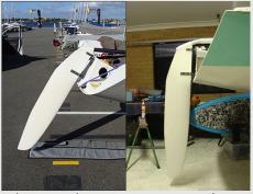
The adapter kit includes a new rudder bracket to replace your current one (see photo below) plus an angled tiller so you can use your existing rudder.
